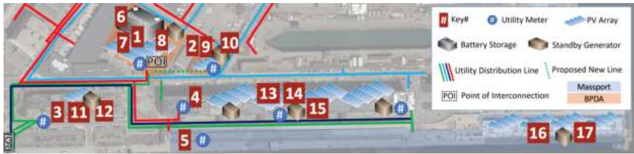
Fig. 3.2: RLFMP Microgrid - Geospatial Overview
